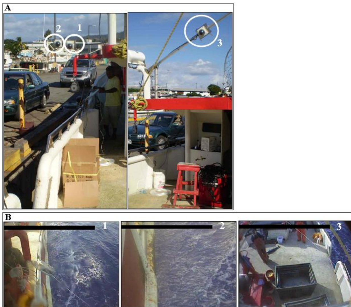
Figure 6. A. Camera installations on the shallow-set vessel S1, two on the fabricated outboard mount, one giving a close-up view of the waterside of the sea door and the other giving a wide angle view of both sides of the rail (left). A third camera is mounted on a rail support and covers the deck inside the sea door (right). B. Example images from the corresponding camera views.
