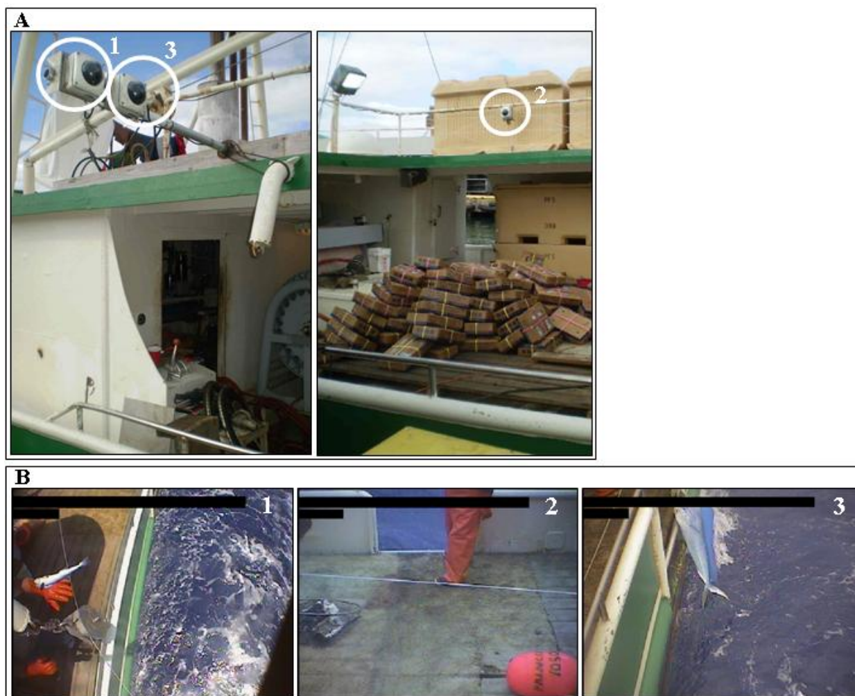
Figure 7. A. Camera installations on the shallow-set vessel S2, two on the fabricated outboard mount, one giving a close-up view of the waterside of the sea door and the other giving a wide angle view of both sides of the rail (left). A third camera is mounted on a rail support and covers the deck inside the sea door (right). B. Example images from the corresponding camera views.
