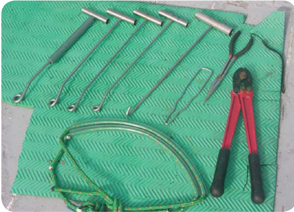
De-hooking and line cutting equipment that can be used to safely release a sea turtle that is accidentally captured during longline fishing operations.
